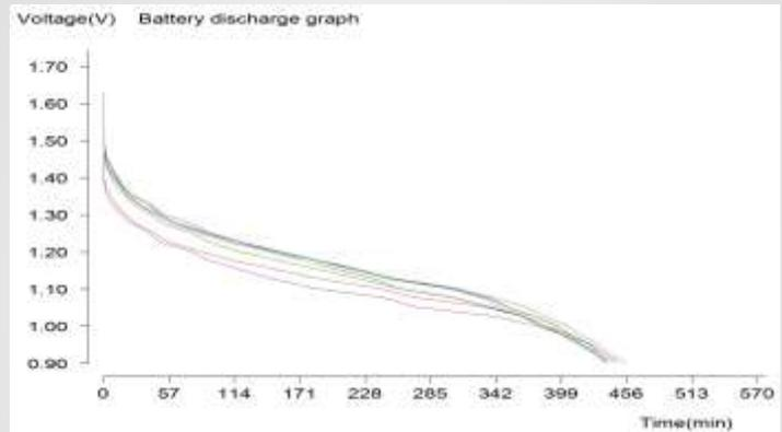
Number of batteries under test: 9
